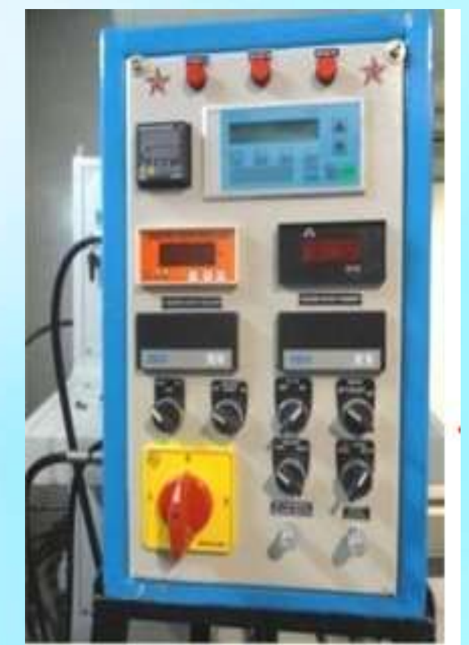
Power Supply and Control Panel for Cold Spray Coating System
