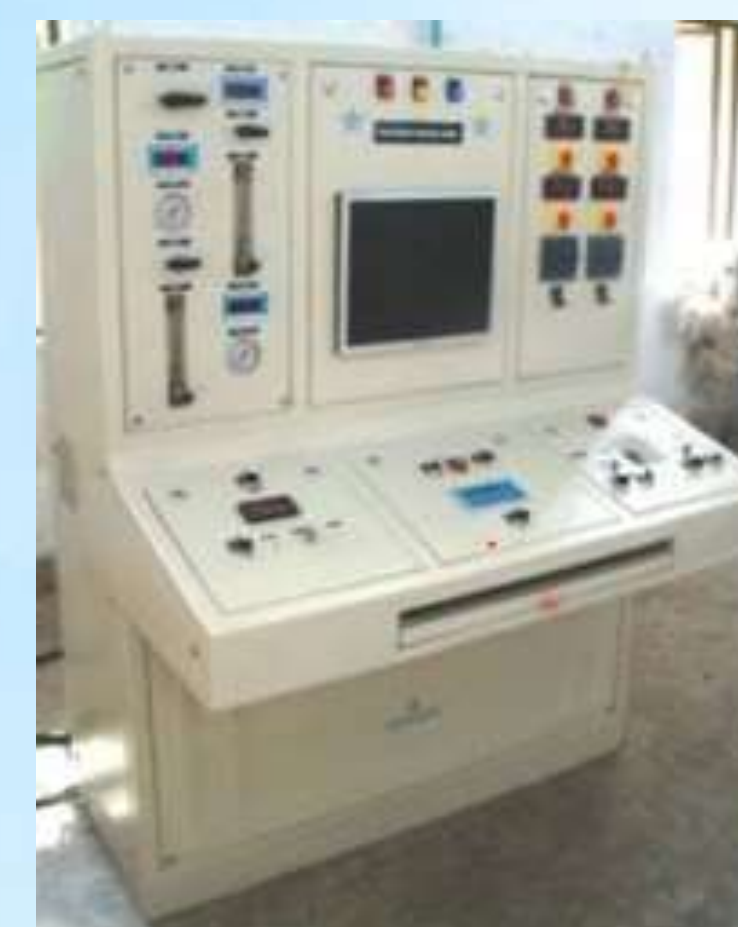
Power Supply and Control Panel for Cold Spray Coating System
