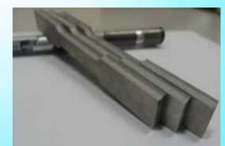
Al Alloy Specimens After Repair
